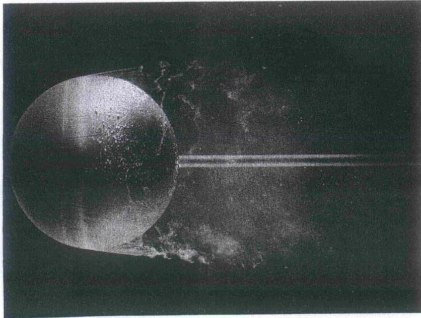
**Figure 15-20** Subcritical flow over a sphere is shown at  $Re = 15,000$ . Laminar separation occurs forward of the equator. Photograph courtesy of H. Werlé, ONERA, Catillon, France.
