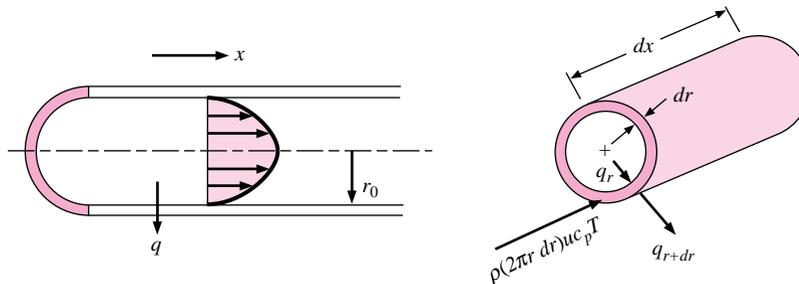
**Figure 5-16** | Force balance on fluid element in tube flow.
