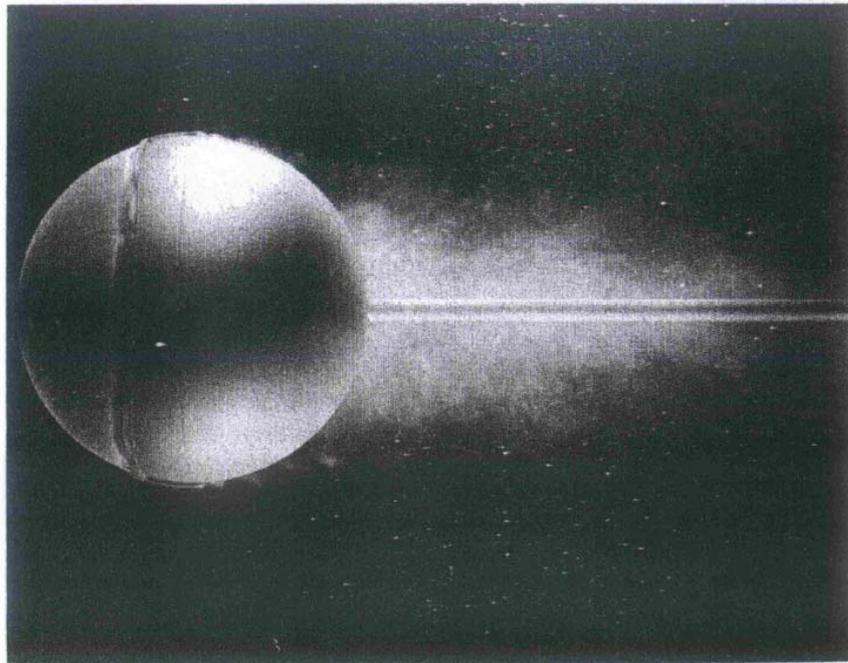
**Figure 15-21** Supercritical flow at  $Re = 30,000$ . Normally this flow is subcritical, but a small trip wire has induced transition to a turbulent boundary layer. Separation is now downstream of the equator, and the wake is smaller. Photograph from ONERA by H. Werlé (1980).
