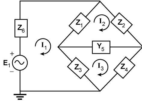
$$\begin{aligned} \underline{I}_1[\underline{Z}_1 + \underline{Z}_3 + \underline{Z}_6] - \underline{Z}_1\underline{I}_2 - \underline{Z}_3\underline{I}_3 &= \underline{E} \\ \underline{I}_2[\underline{Z}_1 + \underline{Z}_2 + \underline{Z}_5] - \underline{Z}_1\underline{I}_1 - \underline{Z}_5\underline{I}_3 &= 0 \\ \underline{I}_3[\underline{Z}_3 + \underline{Z}_4 + \underline{Z}_5] - \underline{Z}_3\underline{I}_1 - \underline{Z}_5\underline{I}_2 &= 0 \end{aligned}$$
