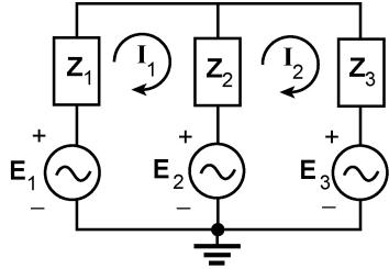
$$\mathbf{Z}_1 = 12 \Omega + j12 \Omega = 16.971 \Omega \angle 45^\circ$$
