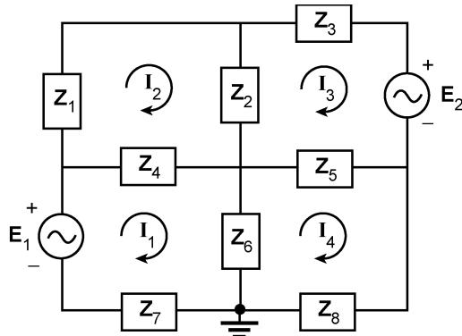
$$\begin{aligned} \mathbf{Z}_1 &= 10 \Omega + j20 \Omega & \mathbf{Z}_2 &= -j20 \Omega \\ \mathbf{Z}_3 &= 80 \Omega \angle 0^\circ & \mathbf{Z}_4 &= 6 \Omega \angle 0^\circ \\ \mathbf{Z}_5 &= 15 \Omega \angle 90^\circ & \mathbf{Z}_6 &= 10 \Omega \angle 0^\circ \\ \mathbf{Z}_7 &= 5 \Omega \angle 0^\circ & \mathbf{Z}_8 &= 5 \Omega - j20 \Omega \\ \mathbf{E}_1 &= 25 \text{ V} \angle 0^\circ & \mathbf{E}_2 &= 75 \text{ V} \angle 20^\circ \end{aligned}$$
