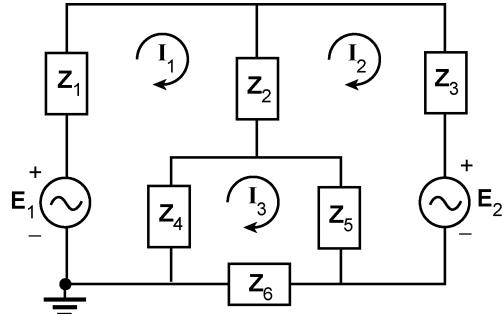
$$\begin{aligned}\mathbf{Z}_1 &= 5 \Omega \angle 0^\circ, \mathbf{Z}_2 = 5 \Omega \angle 90^\circ \\ \mathbf{Z}_3 &= 4 \Omega \angle 0^\circ, \mathbf{Z}_4 = 6 \Omega \angle -90^\circ \\ \mathbf{Z}_5 &= 4 \Omega \angle 0^\circ, \mathbf{Z}_6 = 6 \Omega + j8 \Omega \\ \mathbf{E}_1 &= 20 \text{ V} \angle 0^\circ, \mathbf{E}_2 = 40 \text{ V} \angle 60^\circ\end{aligned}$$
