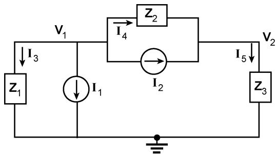
$$\begin{aligned} Z_1 &= 3 \Omega + j4 \Omega = 5 \Omega \angle 53.13^\circ \\ Z_2 &= 2 \Omega \angle 0^\circ \\ Z_3 &= 6 \Omega \angle 0^\circ \parallel 8 \Omega \angle -90^\circ \\ &= 4.8 \Omega \angle -36.87^\circ \\ I_1 &= 0.6 \text{ A} \angle 20^\circ \\ I_2 &= 4 \text{ A} \angle 80^\circ \end{aligned}$$
