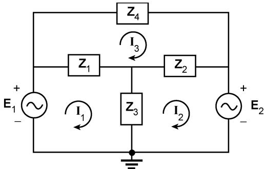
$$\begin{aligned}\mathbf{Z}_1 &= 15 \Omega \angle 0^\circ, \mathbf{Z}_2 = 15 \Omega \angle 0^\circ \\ \mathbf{Z}_3 &= -j10 \Omega = 10 \Omega \angle -90^\circ \\ \mathbf{Z}_4 &= 3 \Omega + j4 \Omega = 5 \Omega \angle 53.13^\circ \\ \mathbf{E}_1 &= 220 \text{ V} \angle 0^\circ \\ \mathbf{E}_2 &= 100 \text{ V} \angle 90^\circ\end{aligned}$$
