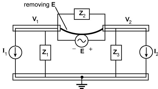
$$\begin{aligned} \mathbf{Z}_1 &= 1 \text{ k}\Omega \angle 0^\circ \\ \mathbf{Z}_2 &= 2 \text{ k}\Omega \angle 90^\circ \\ \mathbf{Z}_3 &= 3 \text{ k}\Omega \angle -90^\circ \\ \mathbf{I}_1 &= 12 \text{ mA } \angle 0^\circ \\ \mathbf{I}_2 &= 4 \text{ mA } \angle 0^\circ \\ \mathbf{E} &= 10 \text{ V } \angle 0^\circ \end{aligned}$$
