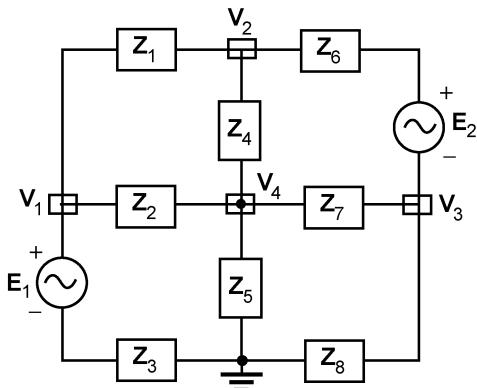
$$\begin{aligned}\mathbf{Z}_1 &= 10 \Omega + j20 \Omega \\ \mathbf{Z}_2 &= 6 \Omega \angle 0^\circ \\ \mathbf{Z}_3 &= 5 \Omega \angle 0^\circ \\ \mathbf{Z}_4 &= 20 \Omega \angle -90^\circ \\ \mathbf{Z}_5 &= 10 \Omega \angle 0^\circ \\ \mathbf{Z}_6 &= 80 \Omega \angle 0^\circ \\ \mathbf{Z}_7 &= 15 \Omega \angle 90^\circ \\ \mathbf{Z}_8 &= 5 \Omega - j20 \Omega\end{aligned}$$
