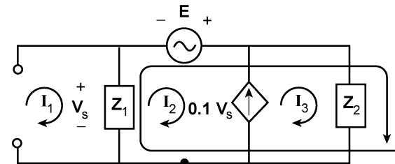
$$\begin{aligned}\mathbf{Z}_1 &= 1 \text{ k}\Omega \angle 0^\circ \\ \mathbf{Z}_2 &= 4 \text{ k}\Omega + j6 \text{ k}\Omega \\ \mathbf{E} &= 10 \text{ V} \angle 0^\circ\end{aligned}$$
