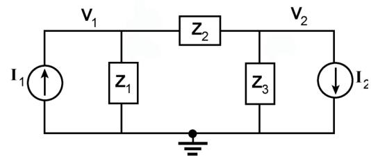
$$\begin{aligned}\mathbf{Z}_1 &= 4 \text{ k}\Omega \angle 0^\circ \\ \mathbf{Z}_2 &= 1 \text{ k}\Omega \angle 90^\circ \\ \mathbf{Z}_3 &= 8 \text{ k}\Omega \angle -90^\circ \\ \mathbf{I}_1 &= 3 \text{ mA} \angle 0^\circ \\ \mathbf{I}_2 &= 5 \text{ mA} \angle 30^\circ\end{aligned}$$
