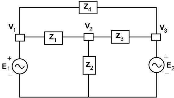
$$\begin{aligned}\mathbf{Z}_1 &= 15 \Omega \angle 0^\circ \\ \mathbf{Z}_2 &= 10 \Omega \angle -90^\circ \\ \mathbf{Z}_3 &= 15 \Omega \angle 0^\circ \\ \mathbf{Z}_4 &= 3 \Omega + j4 \Omega\end{aligned}$$
