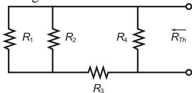
$$\begin{aligned}R_{Th} &= R_4 \parallel (R_3 + R_1 \parallel R_2) \\&= 1 \text{ k}\Omega \parallel (2.7 \text{ k}\Omega + 8.2 \text{ k}\Omega \parallel 2.2 \text{ k}\Omega) \\&= 1 \text{ k}\Omega \parallel 4.43 \text{ k}\Omega \\&= 0.816 \text{ k}\Omega\end{aligned}$$
