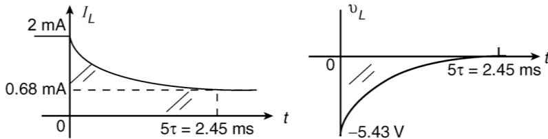
28. a. Steady-state:  $I_L = \frac{8 \text{ V}}{1.5 \text{ k}\Omega} = 5.33 \text{ mA}, V_L = 0 \text{ V}$
