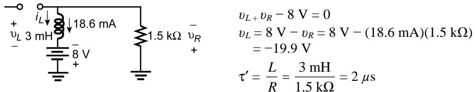
$I_i = 18.6 \text{ mA} \quad I_f = \frac{8 \text{ V}}{1.5 \text{ k}\Omega} = 5.33 \text{ mA}$
