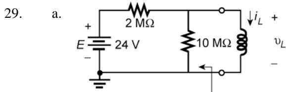
$R_{Th} = 2 \text{ M}\Omega \parallel 10 \text{ M}\Omega = 1.67 \text{ M}\Omega$
