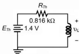
$$\begin{aligned}\tau &= \frac{L}{R} = \frac{10 \text{ mH}}{0.816 \text{ k}\Omega} = 12.25 \mu\text{s} \\v_L &= 1.4 \text{ V} e^{-t/12.25\mu\text{s}} \\&= 1.4 \text{ V} e^{-25\mu\text{s}/12.25\mu\text{s}} \\&= 1.4 \text{ V} e^{-2.05} \\&= 1.4 \text{ V}(128.73 \times 10^{-3}) \\&= \mathbf{180 \text{ mV}}\end{aligned}$$
