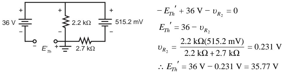
$$\begin{aligned} -E_{Th}' + 36 \text{ V} - v_{R_2} &= 0 \\ E_{Th}' &= 36 - v_{R_2} \\ v_{R_2} &= \frac{2.2 \text{ k}\Omega (515.2 \text{ mV})}{2.2 \text{ k}\Omega + 2.7 \text{ k}\Omega} = 0.231 \text{ V} \\ \therefore E_{Th}' &= 36 \text{ V} - 0.231 \text{ V} = 35.77 \text{ V} \end{aligned}$$
