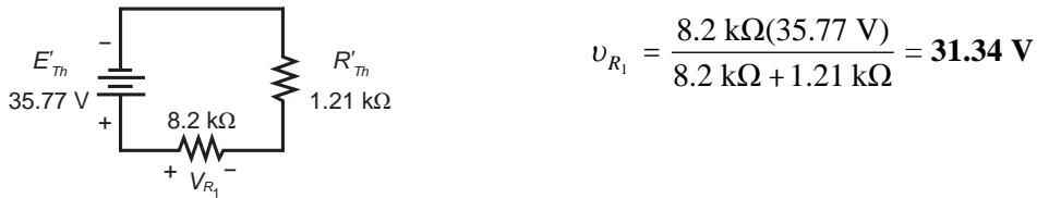
$$v_{R_1} = \frac{8.2 \text{ k}\Omega (35.77 \text{ V})}{8.2 \text{ k}\Omega + 1.21 \text{ k}\Omega} = 31.34 \text{ V}$$
