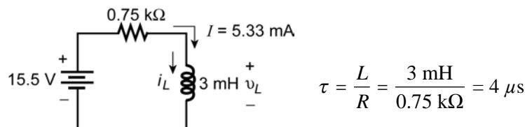
$$I_f = \frac{15.5 \text{ V}}{0.75 \text{ k}\Omega} = 20.67 \text{ mA} \quad I_i = 5.33 \text{ mA}$$
