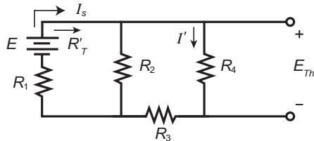
$$\begin{aligned}R'_T &= R_1 + R_2 \parallel (R_3 + R_4) \\&= 8.2 \text{ k}\Omega + 2.2 \text{ k}\Omega \parallel (2.7 \text{ k}\Omega + 1 \text{ k}\Omega) \\&= 8.2 \text{ k}\Omega + 2.2 \text{ k}\Omega \parallel 3.7 \text{ k}\Omega \\&= 8.2 \text{ k}\Omega + 1.38 \text{ k}\Omega \\&= 9.58 \text{ k}\Omega\end{aligned}$$
