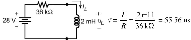
$$i_L = \frac{E}{R}(1 - e^{-t/\tau}) = \frac{28 \text{ V}}{36 \text{ k}\Omega}(1 - e^{-t/\tau}) = 0.778 \text{ mA} (1 - e^{-t/55.56\text{ns}})$$
