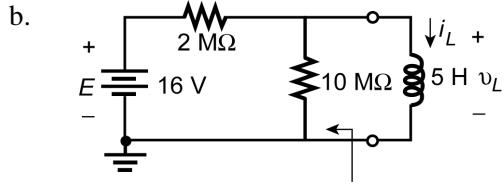
$$R_{Th} = 2 \text{ M}\Omega \parallel 10 \text{ M}\Omega = 1.67 \text{ M}\Omega$$
