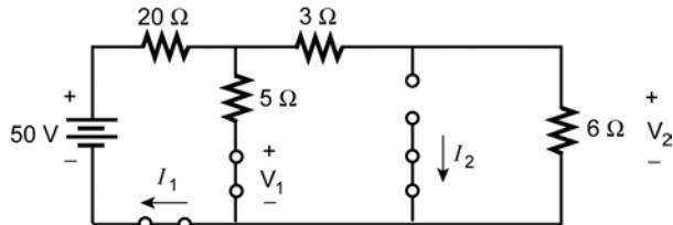
$$V_2 = \frac{6 \Omega(50 \text{ V})}{6 \Omega + 20 \Omega + 3 \Omega} = \mathbf{10.34 \text{ V}}$$
