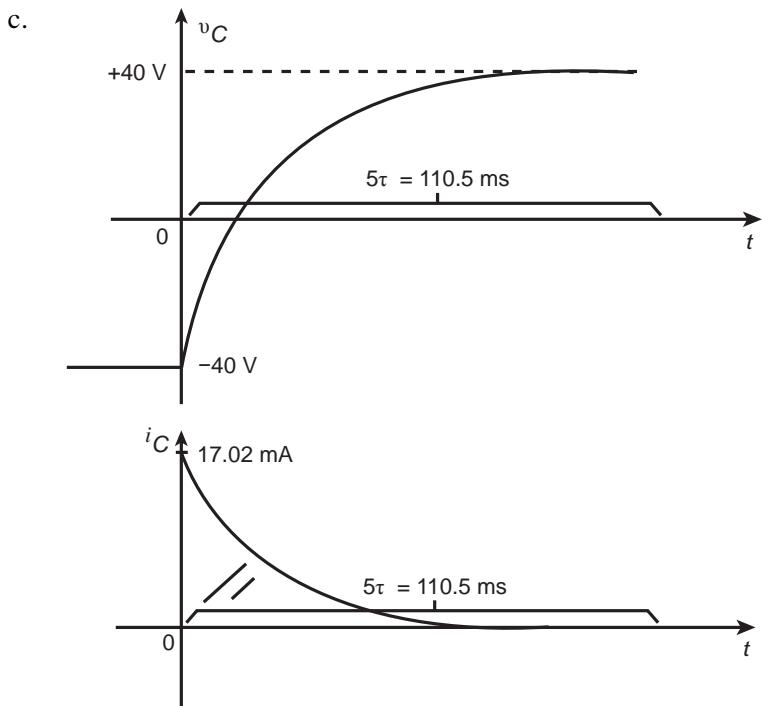
31. a.  $\tau = RC = (4.7 \text{ k}\Omega)(4.7 \mu\text{F}) = 22.1 \text{ ms}$ ,  $V_f = 40 \text{ V}$ ,  $V_i = 40 \text{ V}$
