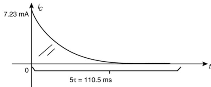
30. a.  $\tau = RC = (4.7 \text{ k}\Omega)(4.7 \mu\text{F}) = 22.1 \text{ ms}, V_f = 40 \text{ V}, V_i = -40 \text{ V}$
