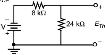
$$E_{Th} = \frac{-24 \text{ k}\Omega (20 \text{ V})}{24 \text{ k}\Omega + 8 \text{ k}\Omega} = -15 \text{ V}$$
