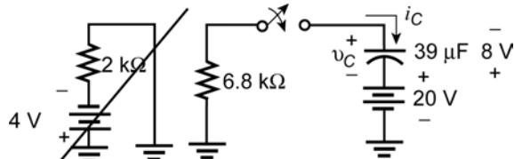
$$\tau = RC = (6.8 \text{ k}\Omega)(39 \mu\text{F}) = 265.2 \text{ ms}$$
