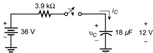
$$\tau = RC = (3.9 \text{ k}\Omega)(18 \mu\text{F}) = 70.2 \text{ ms}$$
