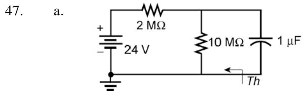
$$R_{Th} = 2 \text{ M}\Omega \parallel 10 \text{ M}\Omega = 1.67 \text{ M}\Omega$$
