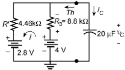
$$R_{Th} = 4.46 \text{ k}\Omega \parallel 6.8 \text{ k}\Omega = 2.69 \text{ k}\Omega$$
