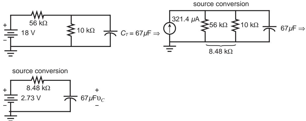
$$\tau = RC = (8.48 \text{ k}\Omega)(67 \mu\text{F}) = 568.2 \text{ ms}$$
