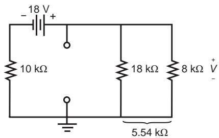
$$V = \frac{5.54 \text{ k}\Omega(18 \text{ V})}{5.54 \text{ k}\Omega + 10 \text{ k}\Omega} = 6.42 \text{ V}$$
