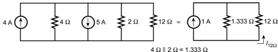
$$I_{12\Omega} = \frac{1.333\Omega(1\text{ A})}{1.333\Omega + 12\Omega} = \mathbf{0.1\text{ A}}$$
