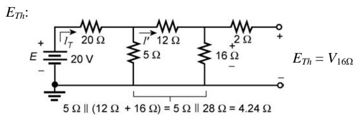
$$I_T = \frac{20 \text{ V}}{20 \Omega + 4.24 \Omega} = 825.08 \text{ mA}$$
