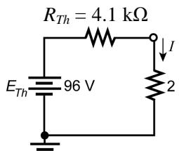
$$\begin{aligned} I &= \frac{96 \text{ V}}{6.1 \text{ k}\Omega} = 15.74 \text{ mA} \\ P &= I^2 R = (15.74 \text{ mA})^2 2 \text{ k}\Omega = \mathbf{0.495 \text{ W}} \\ R &= 100 \text{ k}\Omega: \\ I &= \frac{96 \text{ V}}{104.1 \text{ k}\Omega} = 0.922 \text{ mA} \\ P &= I^2 R = (0.922 \text{ mA})^2 100 \text{ k}\Omega = \mathbf{85 \text{ mW}} \end{aligned}$$
