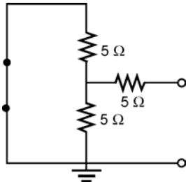
$$\leftarrow R_{Th} = 5 \Omega + 5 \Omega \parallel 5 \Omega = \mathbf{7.5 \Omega}$$
