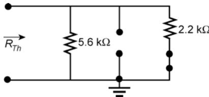
$$R_{Th} = 5.6 \text{ k}\Omega \parallel 2.2 \text{ k}\Omega = 1.58 \text{ k}\Omega$$
