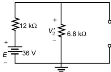
$$V'_2 = \frac{6.8 \text{ k}\Omega(36 \text{ V})}{6.8 \text{ k}\Omega + 12 \text{ k}\Omega} = 13.02 \text{ V}$$
