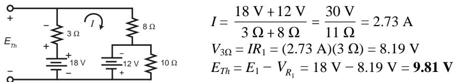
$$I = \frac{18 \text{ V} + 12 \text{ V}}{3 \Omega + 8 \Omega} = \frac{30 \text{ V}}{11 \Omega} = 2.73 \text{ A}$$
