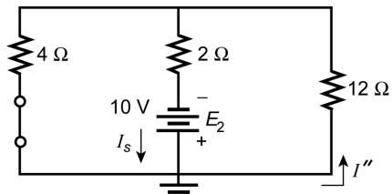
$$R_T \text{ (from source)} = 2\Omega + 4\Omega \parallel 12\Omega \\ = 2\Omega + 3\Omega \\ = 5\Omega$$
