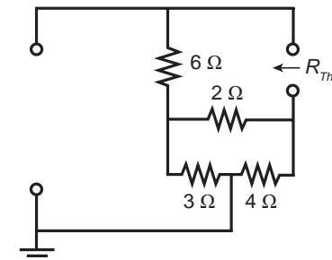
$$R_{Th} = 6 \Omega + 2 \Omega \parallel 7 \Omega = 6 \Omega + 1.56 \Omega = 7.56 \Omega$$
