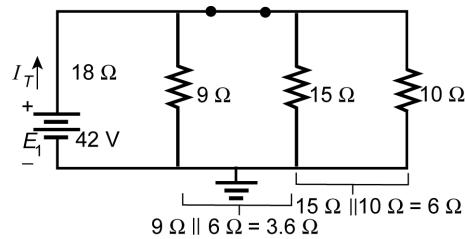
$$I_T = \frac{42 \text{ V}}{18 \Omega + 3.6 \Omega} = 1.944 \text{ A}$$
