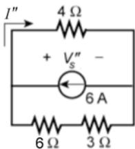
$$I'' = \frac{9 \Omega(6 \text{ A})}{9 \Omega + 4 \Omega} = 4.154 \text{ A}$$
