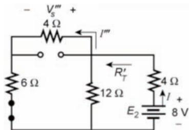
$$I = \frac{E_2}{R_T} = \frac{8 \text{ V}}{4 \Omega + 5.455 \Omega} = 0.846 \text{ A}$$
