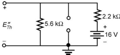
$$\begin{aligned} E''_{Th} &= \frac{5.6 \text{ k}\Omega(16 \text{ V})}{5.6 \text{ k}\Omega + 2.2 \text{ k}\Omega} \\ &= 11.49 \text{ V} \end{aligned}$$
