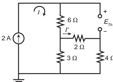
$$\begin{aligned} I &= 2 \text{ A} \\ I' &= \frac{3 \Omega(2 \text{ A})}{3 \Omega + 6 \Omega} = 0.667 \text{ A} \end{aligned}$$
