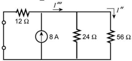
$$R_T = 12 \Omega + 24 \Omega \parallel 56 \Omega = 28.8 \Omega$$
