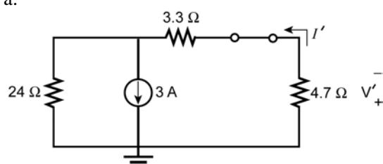
$$I' = \frac{24\Omega(3\text{ A})}{24\Omega + 8\Omega} = 2.25\text{ A}$$
