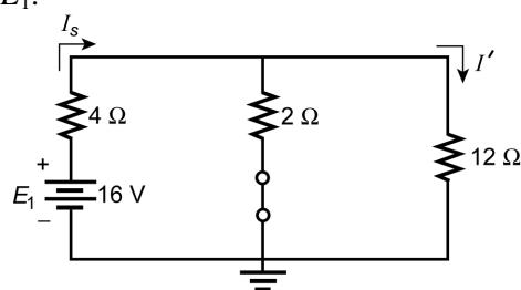
$$R_T \text{ (from source)} = 4\Omega + 2\Omega \parallel 12\Omega \\ = 4\Omega + 1.71\Omega \\ = 5.71\Omega$$
