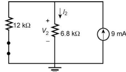
$$I_2 = \frac{12 \text{ k}\Omega(9 \text{ mA})}{12 \text{ k}\Omega + 6.8 \text{ k}\Omega} = 5.75 \text{ mA}$$
