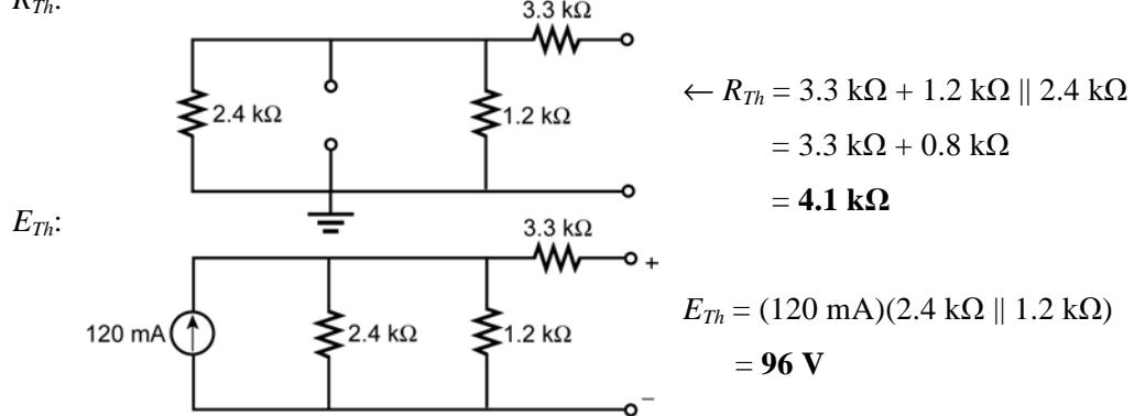
$$\begin{aligned} \leftarrow R_{Th} &= 3.3 \text{ k}\Omega + 1.2 \text{ k}\Omega \parallel 2.4 \text{ k}\Omega \\ &= 3.3 \text{ k}\Omega + 0.8 \text{ k}\Omega \\ &= \mathbf{4.1 \text{ k}\Omega} \end{aligned}$$
