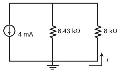
$$I = \frac{6.43 \text{ k}\Omega(4 \text{ mA})}{6.43 \text{ k}\Omega + 8 \text{ k}\Omega} = 1.78 \text{ mA}$$
