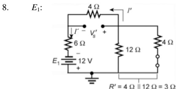
$$I' = \frac{12 \text{ V}}{12 \Omega \parallel 4 \Omega + 4 \Omega + 6 \Omega}$$
