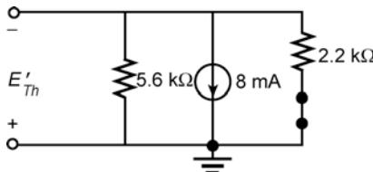
$$\begin{aligned} E'_{Th} &= IR_T \\ &= 8 \text{ mA}(5.6 \text{ k}\Omega \parallel 2.2 \text{ k}\Omega) \\ &= 8 \text{ mA}(1.579 \text{ k}\Omega) \\ &= 12.64 \text{ V} \end{aligned}$$
