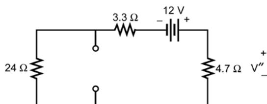
$$V'' = \frac{4.7\Omega(12\text{ V})}{4.7\Omega + 3.3\Omega + 24\Omega} = 1.763\text{ V}$$
