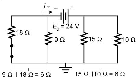
$$I_T = \frac{E_2}{R_T} = \frac{24 \text{ V}}{12 \Omega} = 2 \text{ A}$$
