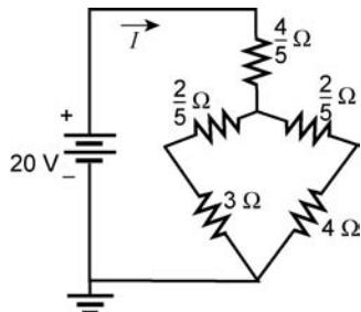
$$I = \frac{20 \text{ V}}{\frac{4}{5} \Omega + \left[ \frac{2}{5} \Omega + 3 \Omega \right] \parallel \left[ \frac{2}{5} \Omega + 4 \Omega \right]}$$
