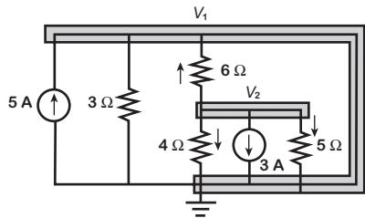
b.  $V_1 = 0 \text{ V}$  (tied to ground)
