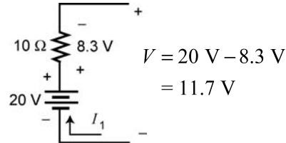
$$I_s = \frac{V}{R_s} = \frac{11.70 \text{ V}}{10 \Omega} = 1.17 \text{ A}$$
