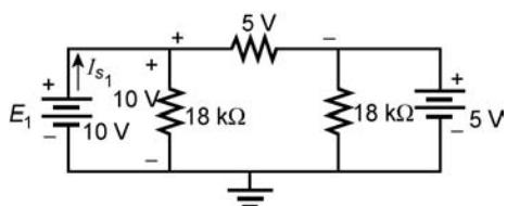
$$I_{s1} = \frac{10 \text{ V}}{18 \text{ k}\Omega} + \frac{5 \text{ V}}{18 \text{ k}\Omega} = \frac{15 \text{ V}}{18 \text{ k}\Omega} = \mathbf{0.83 \text{ mA}}$$
