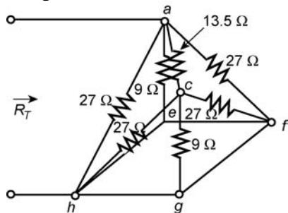
$$c - g: 27 \Omega \parallel 9 \Omega \parallel 27 \Omega = 5.4 \Omega$$
