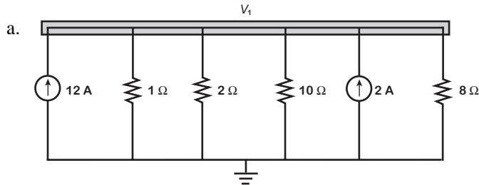
$$V_1 \left[ \frac{1}{1\Omega} + \frac{1}{2\Omega} + \frac{1}{10\Omega} + \frac{1}{8\Omega} \right] = 14 \text{ A}$$
